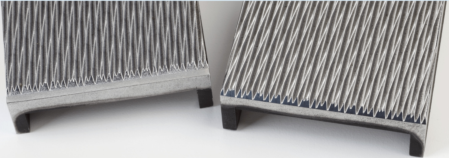
Industrial die, printed using LPBF
